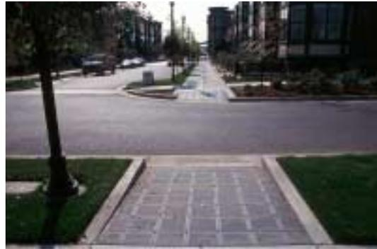
*People walk the way they sit in a vehicle, side by side. Thus, the minimum width for a comfortable sidewalk is 5 feet. Nothing less will do. The eight-foot sidewalk above is more comfortable yet. Ramps are the full width of the sidewalk. Corner radii keep turning speeds low, crossings safe. Research for pedestrians and bicyclists is not measured by saturation (LOS), but by comfort.*
