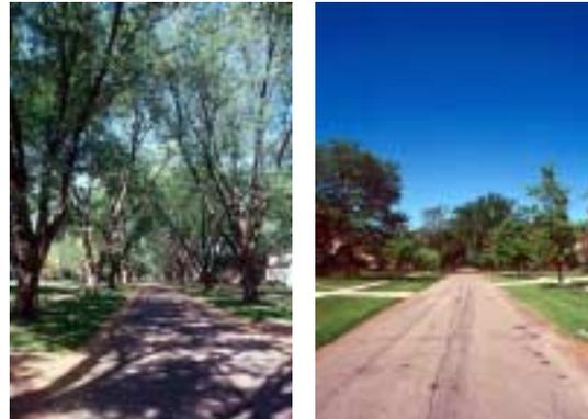
*These two scenes are of the same street in Birmingham, Michigan. The street section with trees produces speeds of about 20 mph. The one without trees produces speeds 10-15 mph faster. Greater safety is achieved with lower speeds and added reaction time. More research is needed on the positive effects of street trees on safety, pavement life, aesthetics, and increased property values.*
